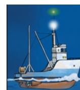
fishing vessel engaged in trawling, two all-round lights in a vertical line, the upper green and the lower white
