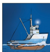
Anchored, after sunset and before sunrise, showing an all-round white light
