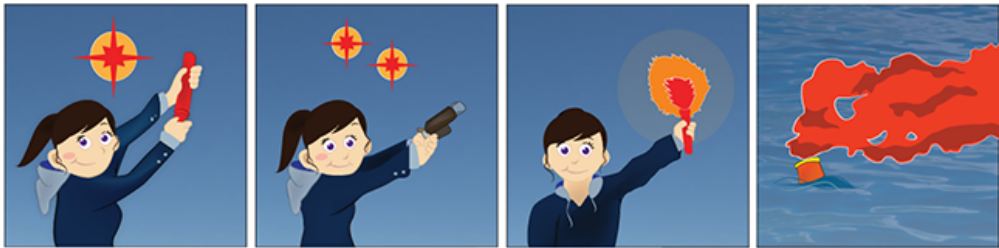
1-Rocket parachute flare 2- Multi star flare 3- Hand-held flare 4- Buoyant or hand smoke signal flare
