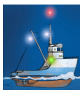
while under way, at night with all-round lights sidelights and one all-round red light
